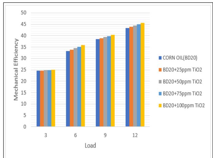
Figure 5: Mechanical Efficiency varying with an increase in load. Source: Authors, (2024).
