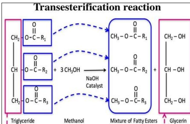
Figure 1: Transesterification process.
