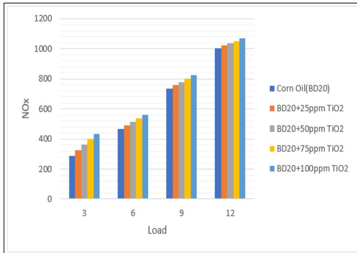
Figure 10: NO<sub>x</sub> varying with an increase in load.
