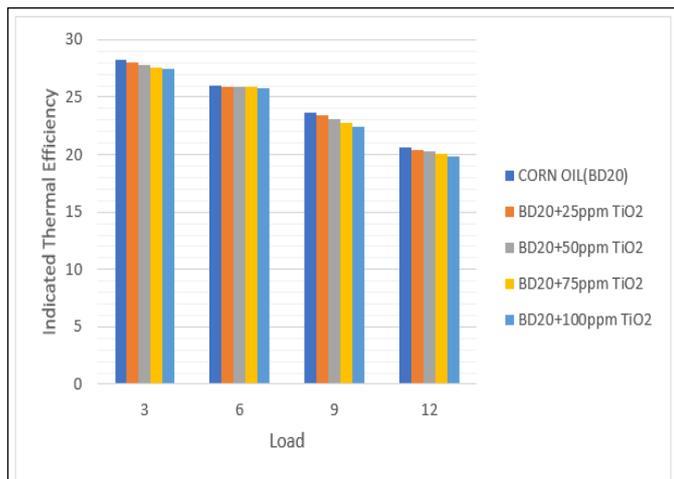
Figure 7: Indicated Thermal Efficiency varying with an increase in load. Source: Authors, (2024).
