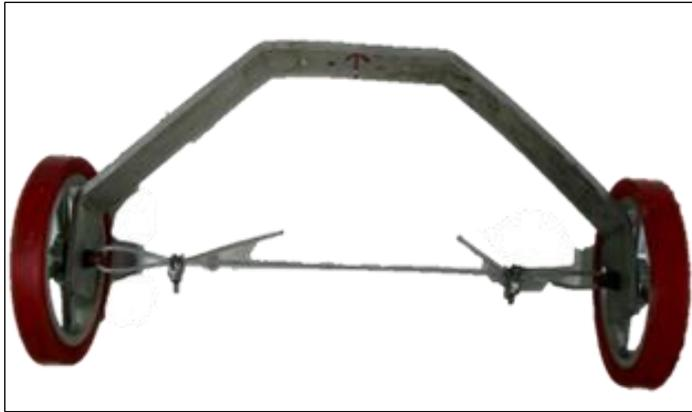
Figure 2: Current landing gear.
