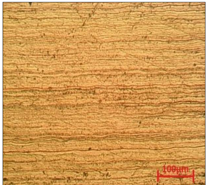
Figure 1.a: ASS-316 base metals' microstructure. Source: Authors, (2024).
