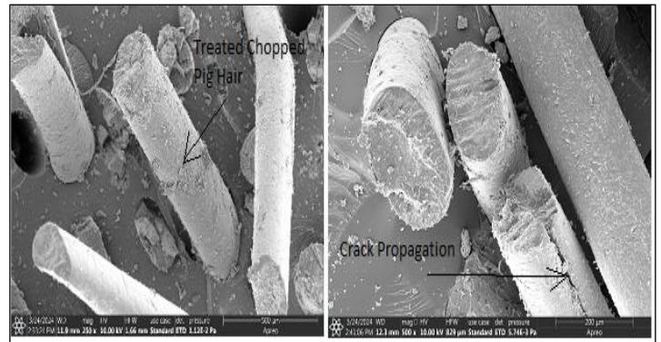
Figure 9: SEM: Bonding between the Treated Chopped Keratin Fiber with epoxy polymer. Source: Authors, (2024).
