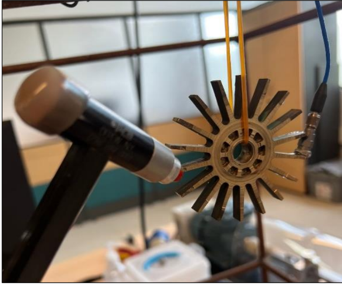
Figure 6: Dynamic vibration test on blades. Source: Authors, (2024).
