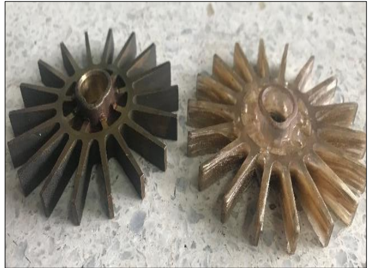
Figure 4: Fabricated impeller and conventional impeller. Source: Authors, (2024).
