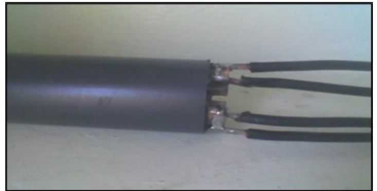
Figure 11: Augmented Rail Launcher Wiring. Source: Authors, (2024).
