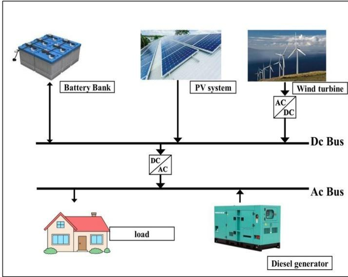
Figure 3: Components of a HMS.
