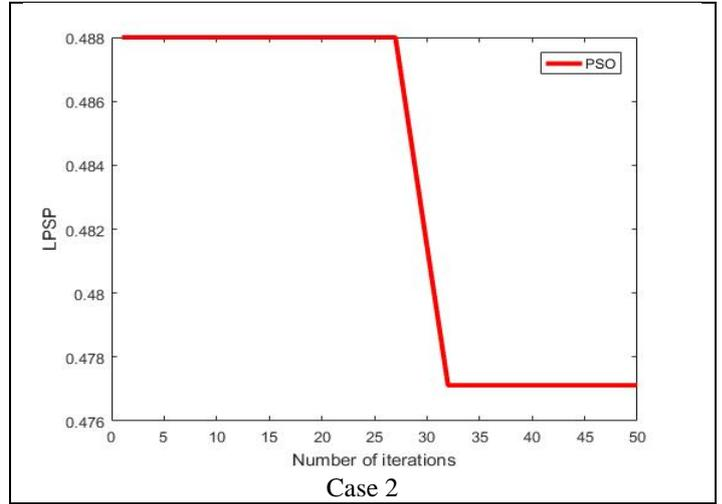
Figure 11: convergence curves for the Loss of power supply probability (LPSP)
