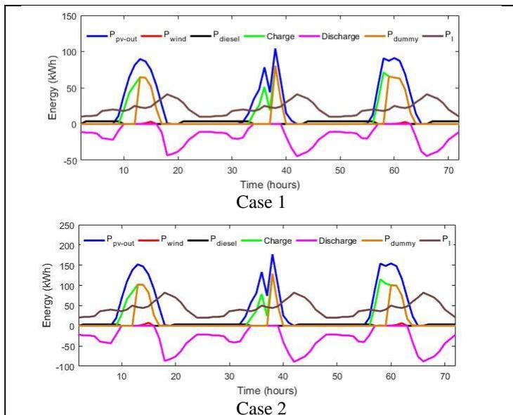
Figure 17: Microgrid system's power over 72 hours using PSO
