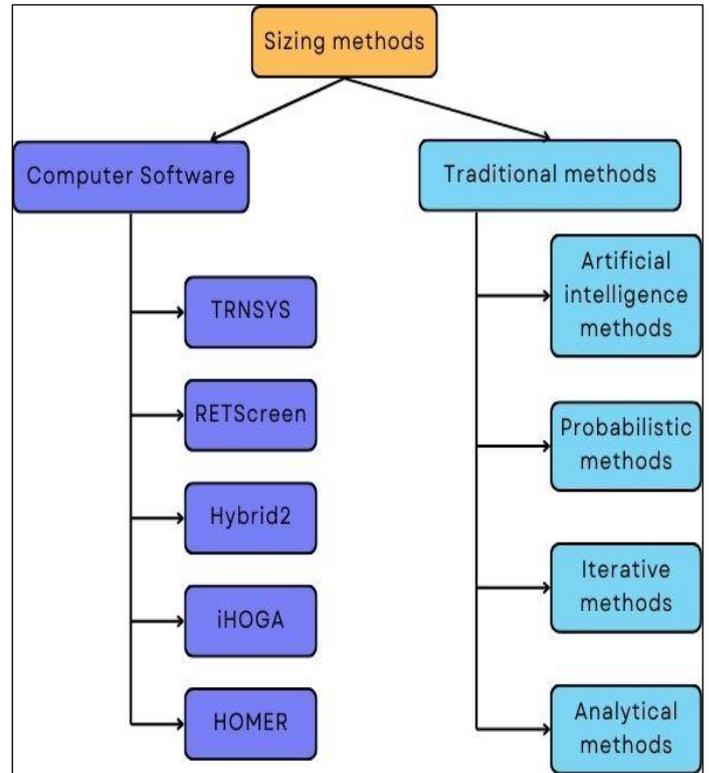
Figure 1: Sizing methods for hybrid system.
