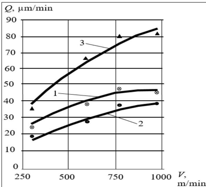
Figure 13: Dependence of the process productivity  $Q$  on the cutting speed  $V$  ( $\Delta Y=$  mm,  $F_R=130$  mm/min) for the CF-FB-0.5 AFIN wheel.
