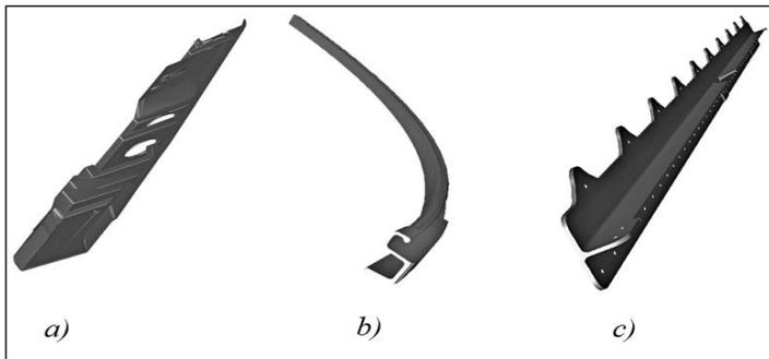
Figure 2: Examples of complex-profile, large-sized aircraft frame parts: a) stringer; b) rim; c) profile. Source: Authors, (2025).
