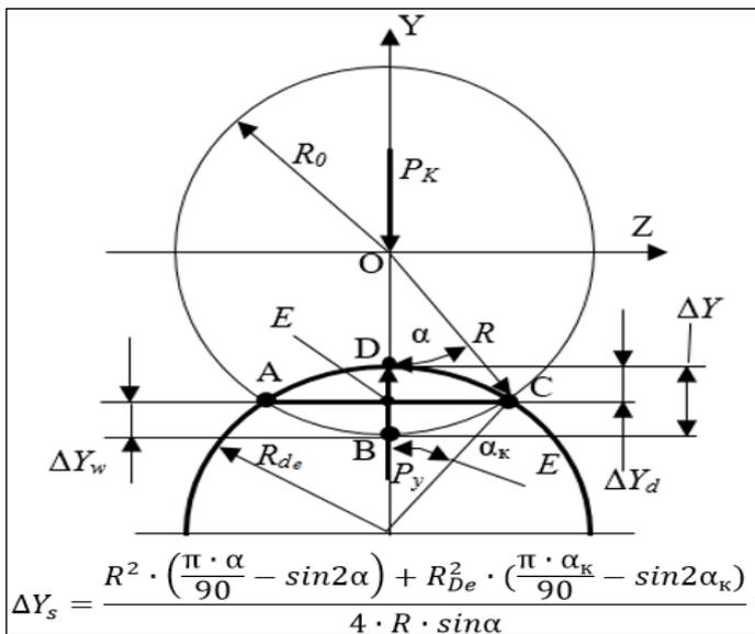
Figure 6: Interaction scheme with a surface rounded along the outer radius. Source: Authors, (2025).
