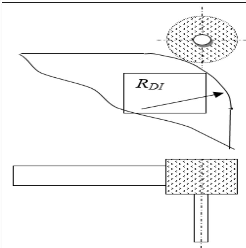
Figure 11: Scheme for processing a surface rounded along the outer radius using an elastic polymer-abrasive wheel.
