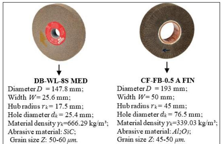
Figure 4: Molded wheel brand DB-WL and flexible wheel consisting of lamellae brand CF-FB. Source: Authors, (2025).
