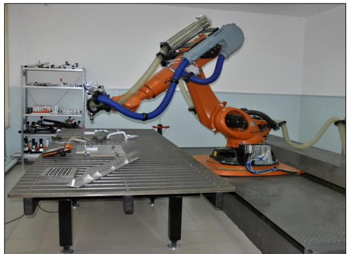
Figure 9: Robotic complex based on KUKA KR 210 R2700 EXTRA industrial robot. Source: Authors, (2025).
