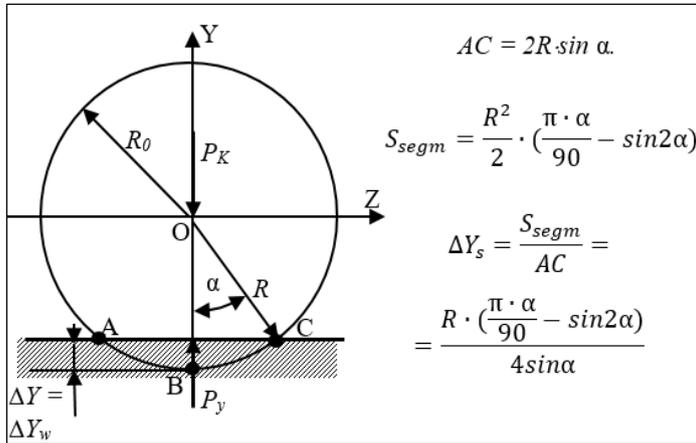
Figure 5: Interaction scheme with a flat surface. Source: Authors, (2025).
