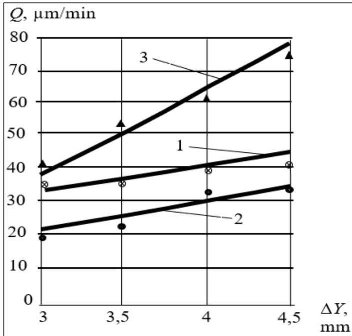
Figure 12: Dependence of the process productivity  $Q$  on deformation  $\Delta Y$  ( $V=606.3$  m/min,  $F_R=130$  mm/min) for the CF-FB-0.5 AFIN wheel.
