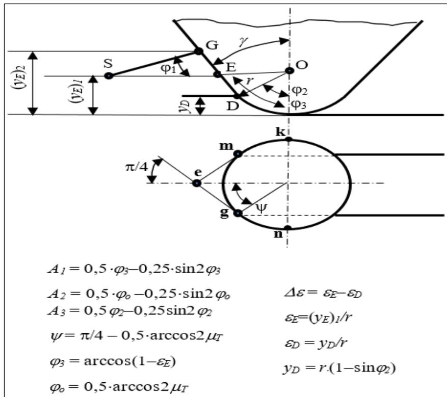
Figure 8: Interaction of a single-grain model with the workpiece surface. Source: Authors, (2025).
