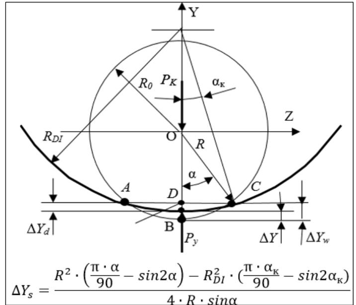
Figure 7: Interaction scheme with a surface rounded along the inner radius.
