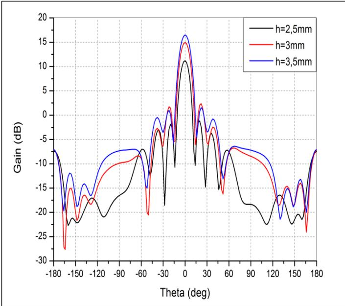
Figure 7: Influence of the concave-shaped form depth on the antenna array gain
