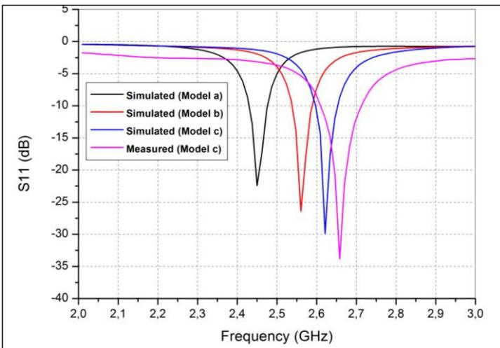
Figure 5: Return loss (S11) for the linear (4x1) microstrip patch antenna array structures. (a) Basic structure. (b) Basic structure with concave-shaped form. (c) Basic structure with concave-shaped form and cut corners. Source: Authors, (2025).
