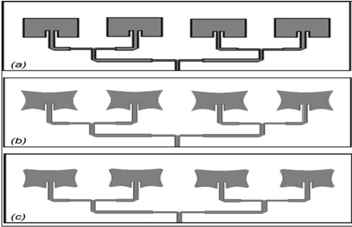
Figure 4: Linear (4x1) microstrip patch antenna array. (a) Basic structure. (b) Basic structure with concave-shaped form. (c) Basic structure with concave-shaped form and cut corners. Source: Authors, (2025).
