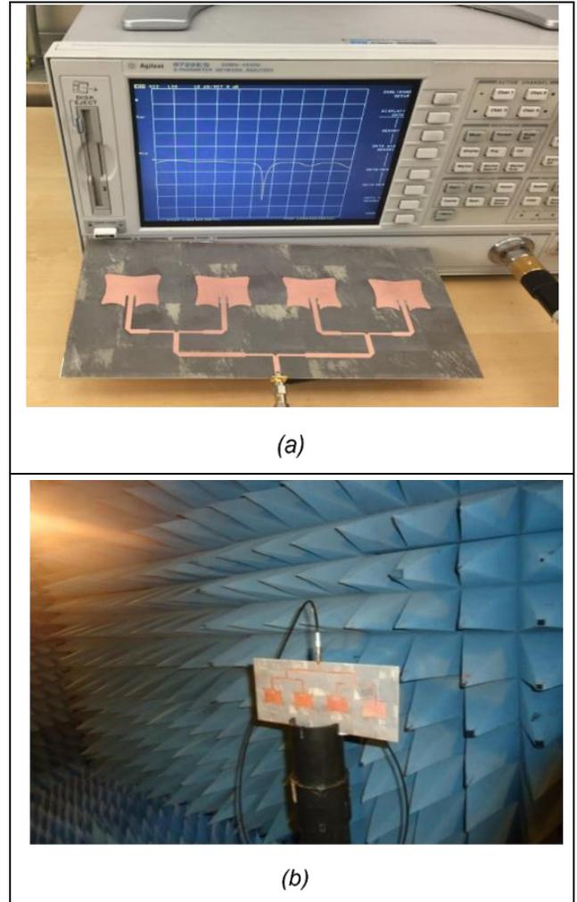
Figure 3: Photograph of the fabricated (4×1) array antenna prototype. (a) S11 parameter measurement protocol with the VNA. (b) Radiation pattern measurement in the anechoic chamber.
