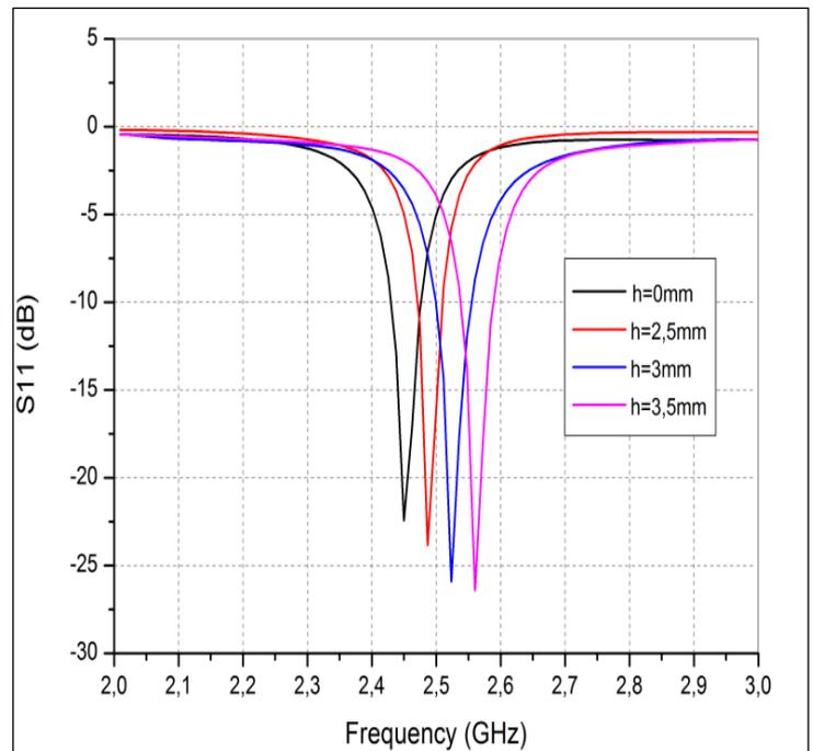
Figure 6: Effect of the concave-shaped form depth on the return loss. Source: Authors, (2025).
