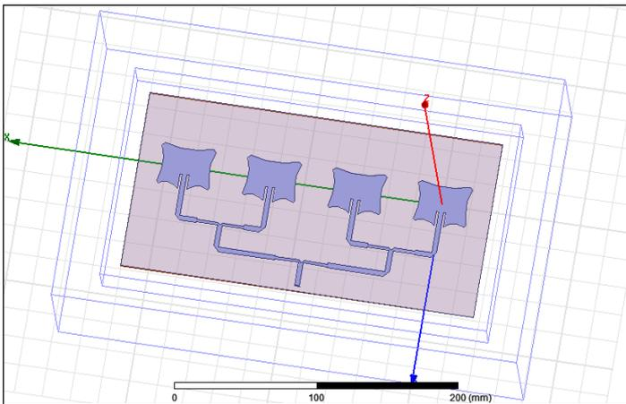
Figure 2: The layout of the proposed (4×1) linear microstrip patch antenna array in HFSS. Source: Authors, (2025).
