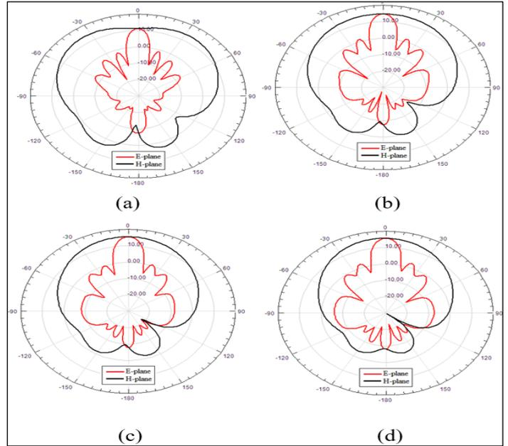
Figure 9: Radiation patterns at 2.45 GHz for the proposed linear patch antenna array. (a)  $h = 2.5\text{mm}$ . (b)  $h = 3\text{mm}$ . (c)  $h = 3.5\text{mm}$ . (d)  $h = 3.5\text{mm}$  and cut corners.
