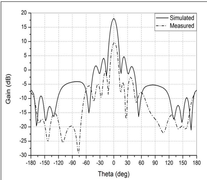
Figure 8: Simulated and measured E-plan gain of the proposed antenna array.
