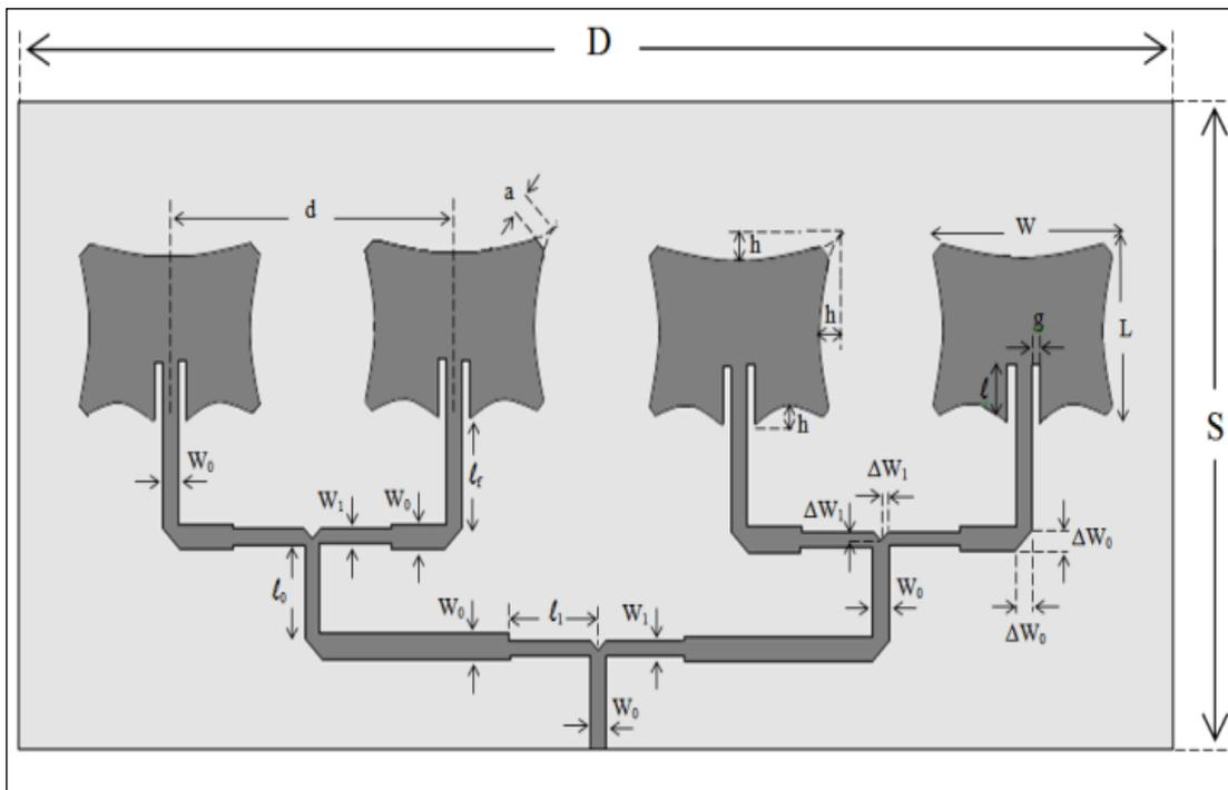
Figure 1: The geometry of the proposed linear microstrip-fed antenna array with four elements. Source: Authors, (2025).
