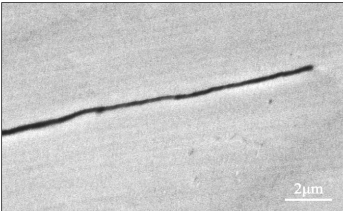
Figure 2: Transgranular stress corrosion cracking. Source: Authors, (2025).
