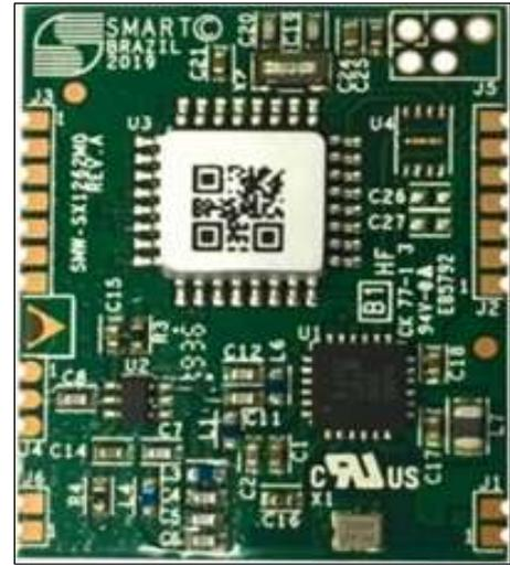
Figure 3: Módulo LoRa®. Source: Iot-Labs, (2024).
