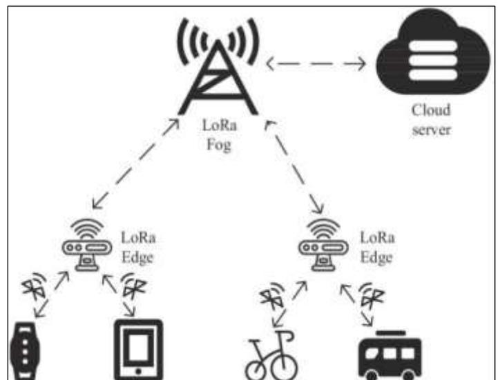
Figure 1: A hybrid LoRa and Bluetooth city network.
