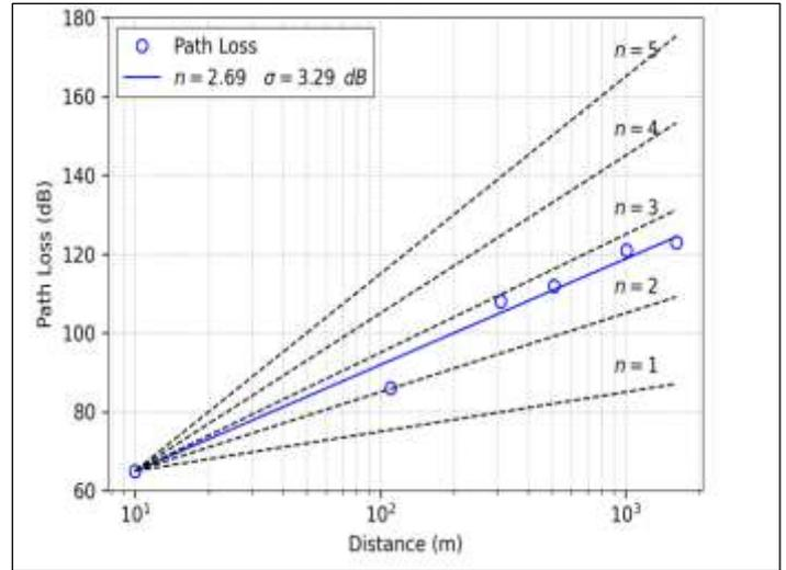
Figure 5: Path Loss as a function of distance.
