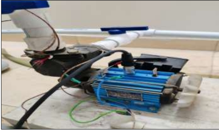
Figure 2: Closer view of a pump with sensors. Source: Authors, (2025).
