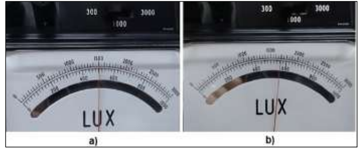
Figure 3: Comparison of the light level on the work plane, a) fluorescent tube, and b) LED tube.
