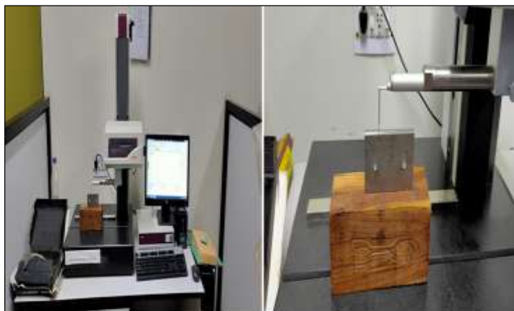
Figure 4: Surface roughness measurement. Source: Authors, (2025).
