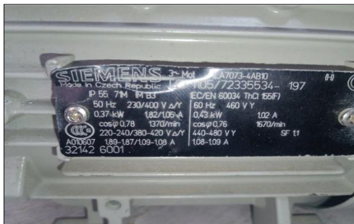
Figure 1: Siemens induction motor nameplate. Source: Authors, (2025).
