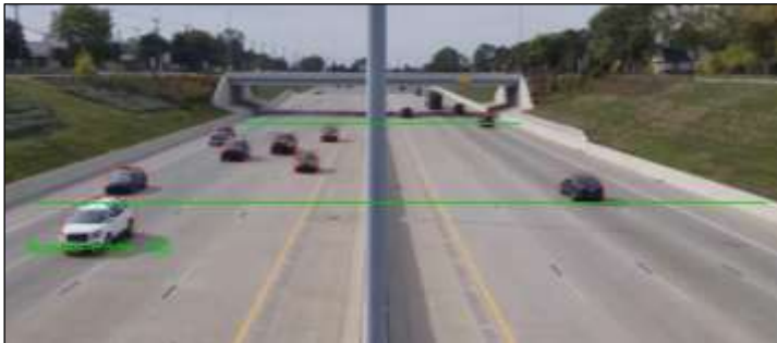
Figure 5: Multi-Vehicle Detection and Tracking Using YOLO and DeepSORT.
