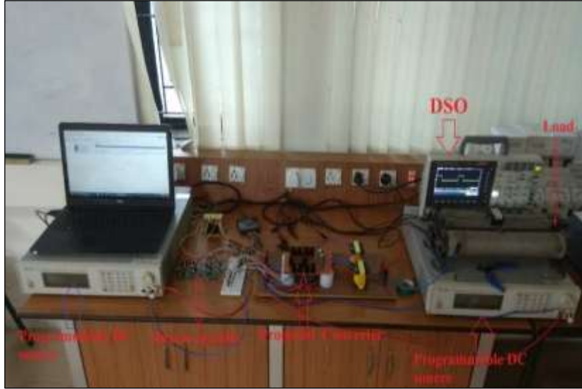
Figure 4: Experimental setup of CUK based novel multi-input converter. Source: Authors, (2025).
