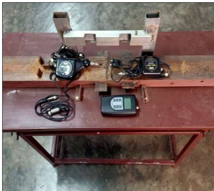
Figure 2: Vibratory Welding Setup.
