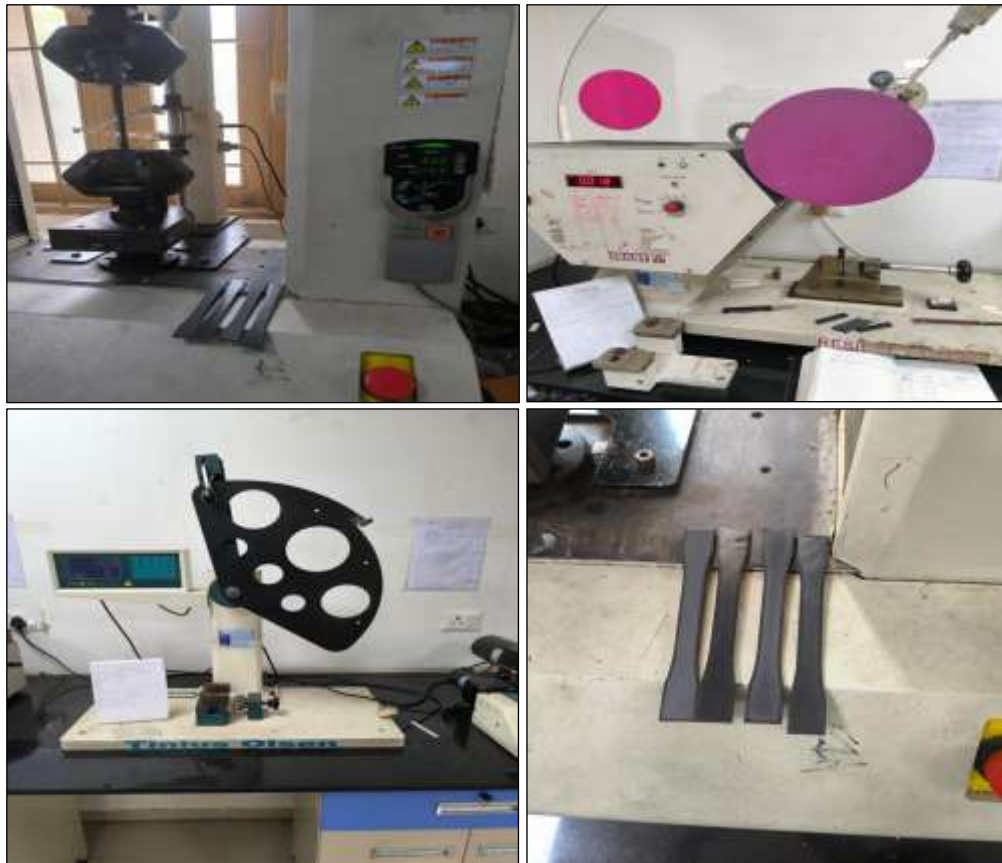
Figure 4: Testing set-up for Specimen of Tensile, Impact and Flexural test.
