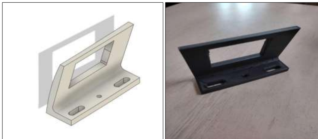
Figure 11: (a) Design of Jig component for LOGO Printing (b) 3D Printing Component.
