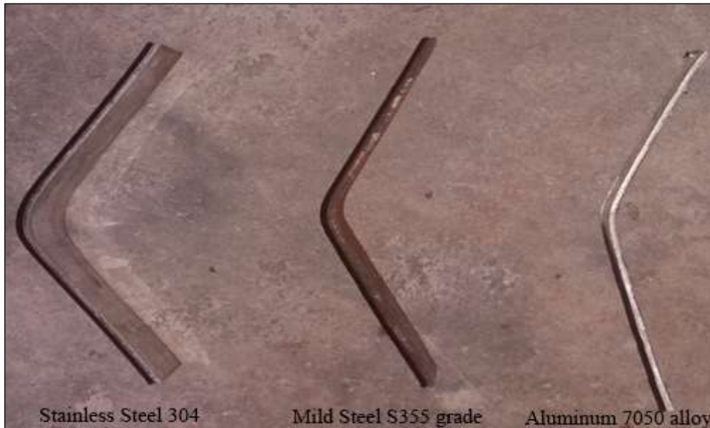
Figure 4: deformed specimens of Stainless Steel 304, Mild Steel S355 grade, and Aluminum 7050 alloy. Source: Authors, (2025).
