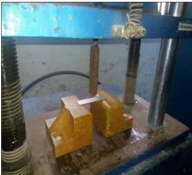
Figure 2: A real view of the experimental setup under a Universal Testing Machine for air-bending. Source: Authors, (2025).
