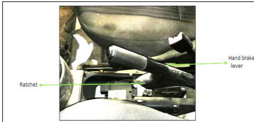
Figure 4: Parking brake lever setup connected in figo vehicle. Source: Authors, (2025).
