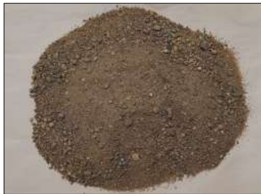
Figure 1: Natural alluvial sand (0–5 mm) used as reference fine aggregate.
