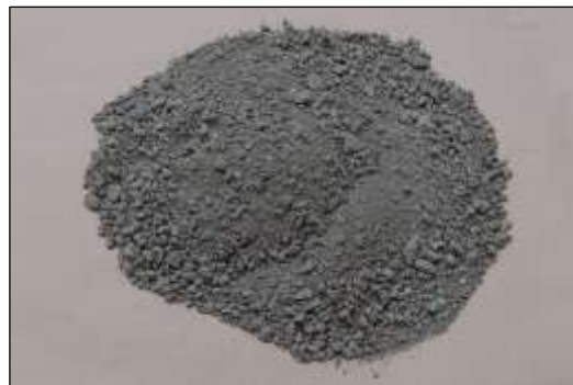
Figure 2: Recycled sand (0–5 mm) produced from processed construction and demolition waste concrete.
