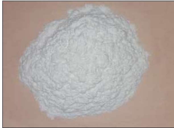
Figure 4: Waste glass powder ( \leq 75 \mu\text{m} ). Source: Authors, (2025).
