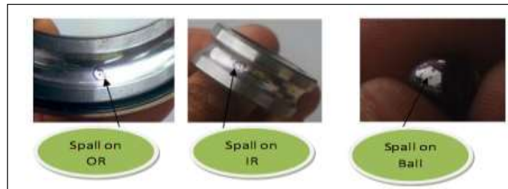
Figure 3: Localized Defect Seeded In Bearing Elements. Source: Authors, (2025).
