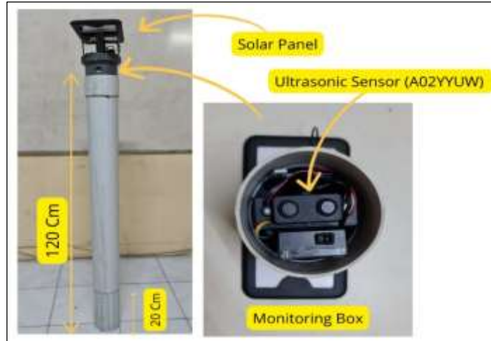
Figure 2: Prototype Hardware Design. Source: Authors, (2025).
