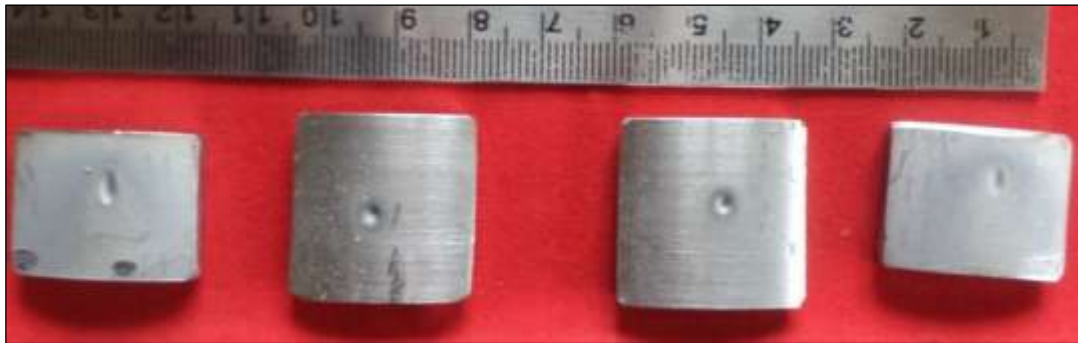
Figure 2: Photograph of specimens eroded at different angles of impact.
