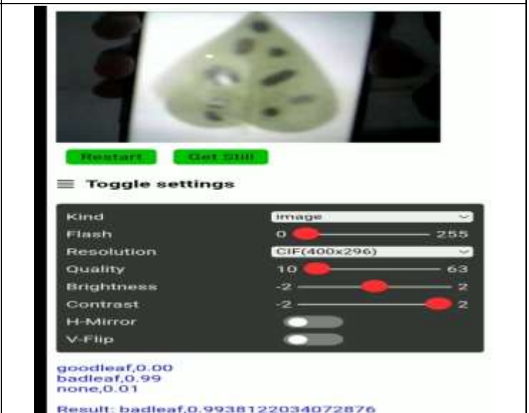
Figure 10: Image analysis result showing leaf classification as bad leaf using multi sensor data fusion with adjustable parameters such as resolution. Source: Authors, (2026).
