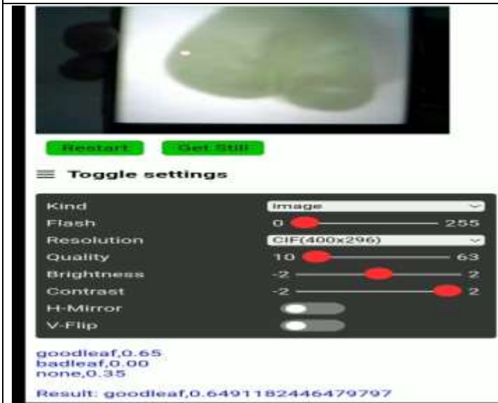
Figure 9: Image analysis result showing leaf classification as good leaf using multi sensor data fusion with adjustable parameters such as resolution, brightness, and contrast. Source: Authors, (2026).
