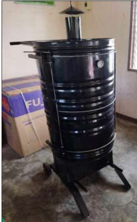
Figure 2: The low-cost and mobile fish smokehouse. Source: Authors (2026).
