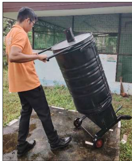
Figure 3: Mobility testing of the fabricated fish smokehouse. Source: Authors (2026).
