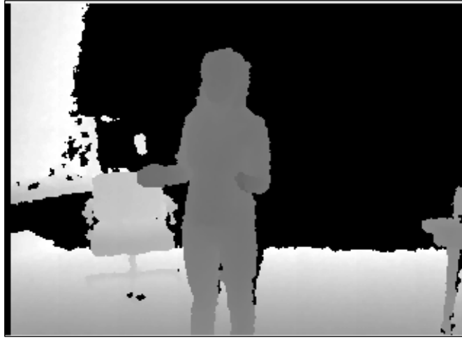
Figure 5: (a) original noisy low resolution Depth Image. Source: Authors, (2026).
