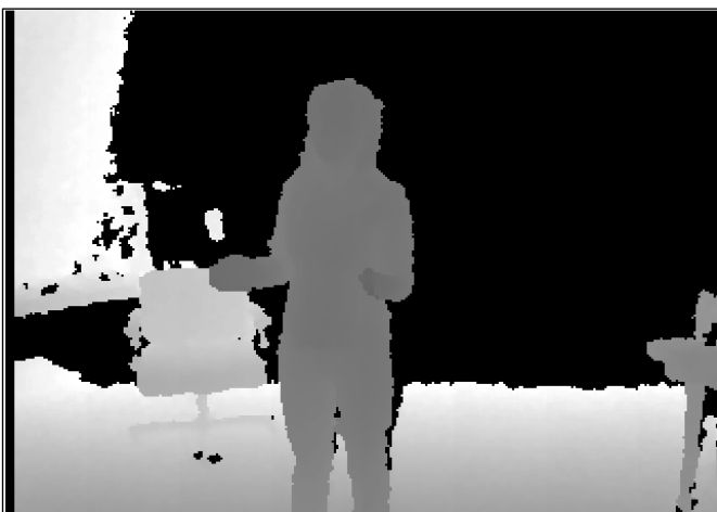
Figure 5: (b) Super resolution Depth Image using Bicubic. Source: Authors, (2026).
