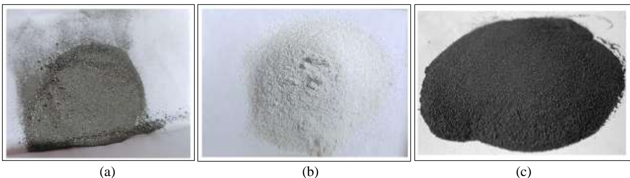
Figure 1: (a) Stainless steel 316, (b) \text{Al}_2\text{O}_3 \text{ ZrO}_2 \text{ Ca}_{10}(\text{PO}_4)_6(\text{OH})_2 , and (c) Silicon.
