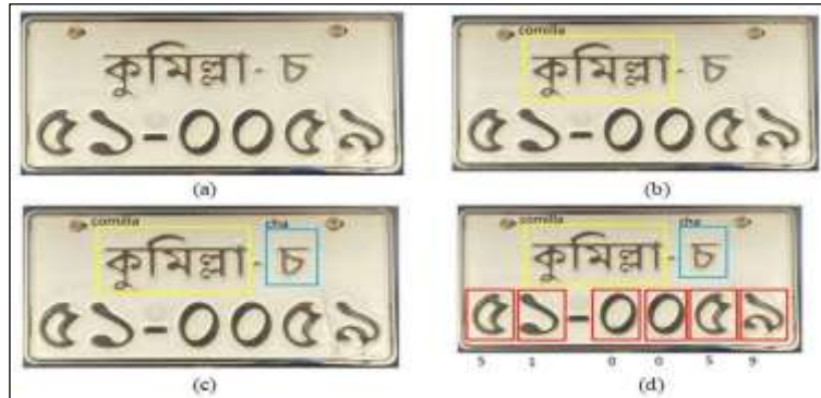
Figure 9: Character Segmentation &amp; Recognition process: (a) image after perspective transformation, (b) city name recognition to text, (c) vehicle type recognition to text and, (d) serial number recognition to text.
