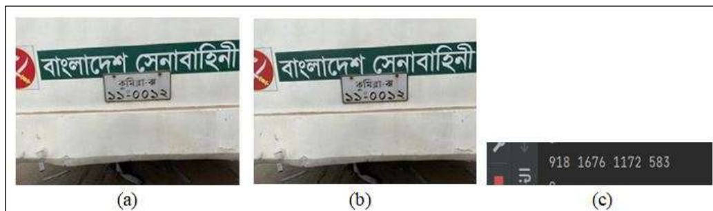
Figure 3: License plate detection: (a) input image, (b) eroded image, and (c) pixel coordinates (x, y, w, h) .
