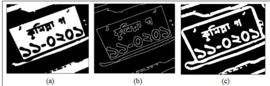
Figure 7: Edge Detection and Adaptive Thresholding: (a) Gaussian blurred image, (b) edge detected image, and (c) image after adaptive thresholding.
