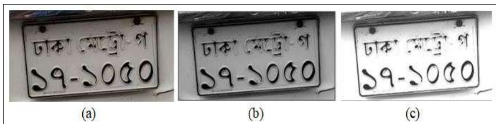
Figure 5: Image gray scaling and brightness increasing: (a) extracted license plate image (RGB image), (b) gray-scale image, and (c) brightness increased gray-scale image.
