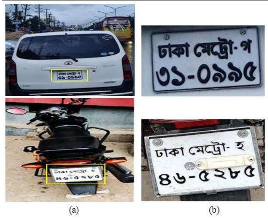
Figure 4: License plate extraction: (a) boundary box drawn images, (b) extracted license plates. Source: Authors, (2026).
