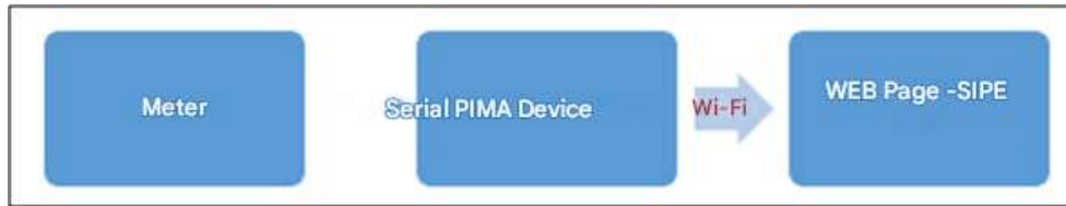
Figure 5: Serial Communication Prototype with WebServer. Source: Authors, (2026).
