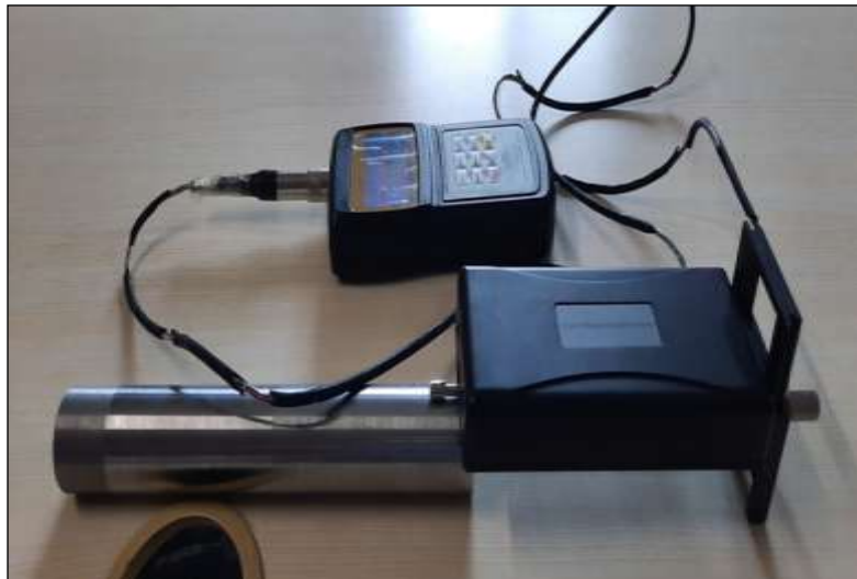
Figure 1: ITI surf test RS 232” (make: ITI, India) surface roughness tester. Source: Authors (2026).
