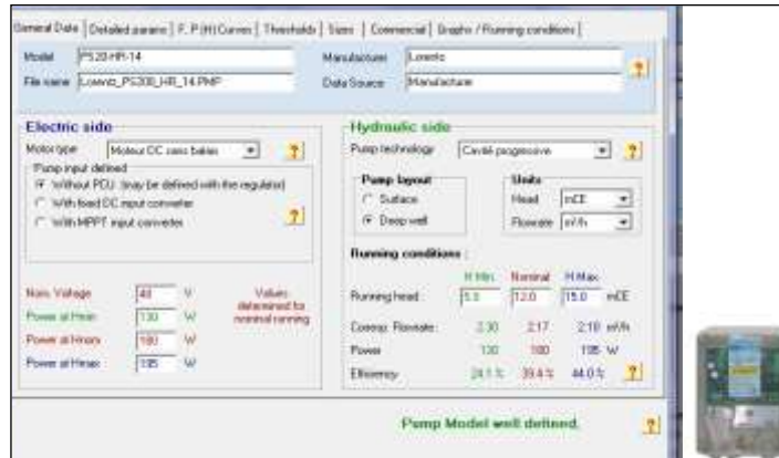
Figure 3: Pump feature PS200_HR-14. Source: Authors, (2026).
