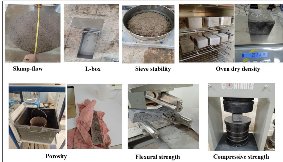
Figure 4: Different tests conducted on fresh and hardened state.
