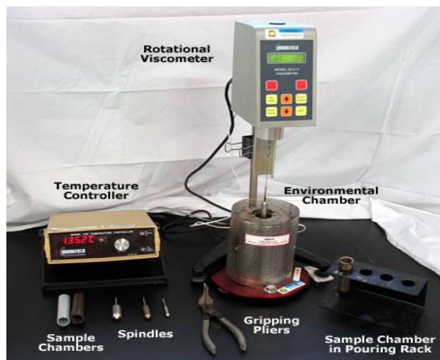
Figure 8: Rotational Viscometer, used for the Brookfield Viscosity Test.
