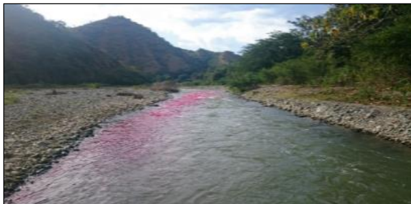
Figure 7: Fluorometric tracer advancing in a river. Source: Authors, (2021).
