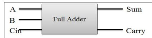
Figure 4: Schematic diagram of full-adder. Source: Authors, (2021).
