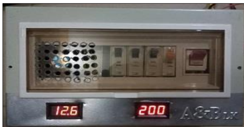
Figure 4: Constructed Hybrid Distribution Board Powered. Source: Authors, (2021).
