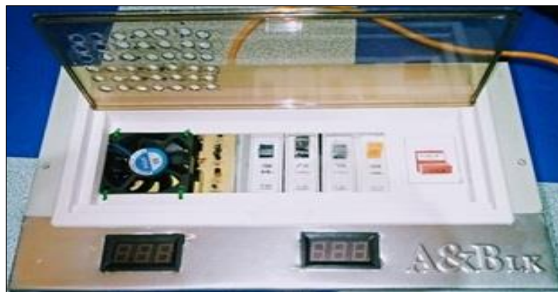
Figure 3: Constructed Hybrid Distribution Board Unpowered. Source: Authors, (2021).
