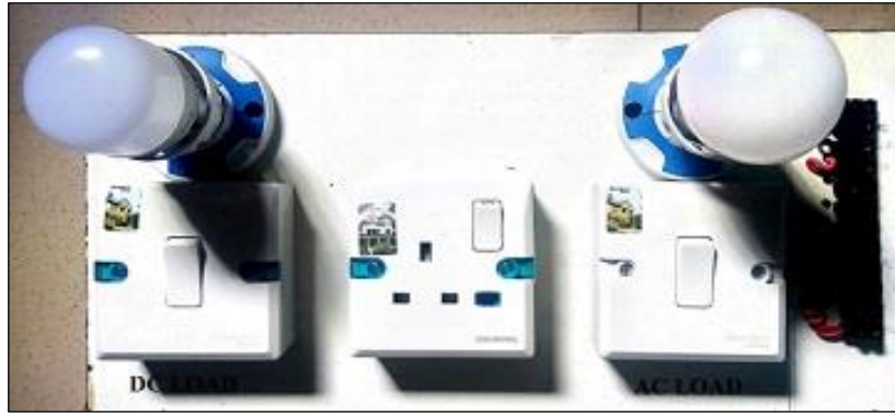
Figure 5: Hybrid Load on Wooden Board when Not Powered. Source: Authors, (2021).
