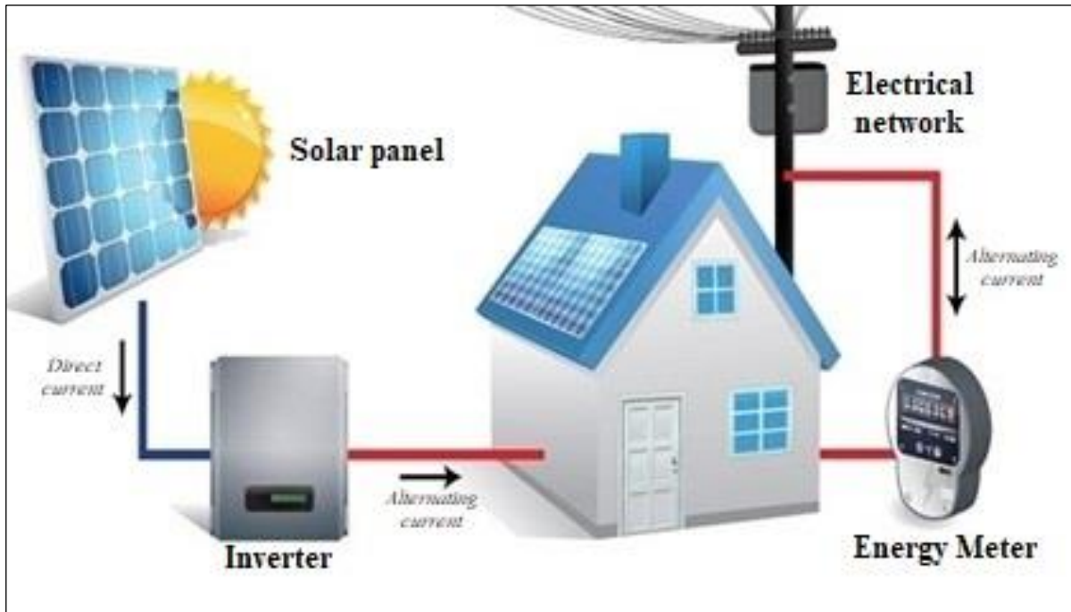
Figure 4: Composition of the photovoltaic solar system connected to the grid. Source: CSR ENERGIA SOLAR, (2008) [39].
