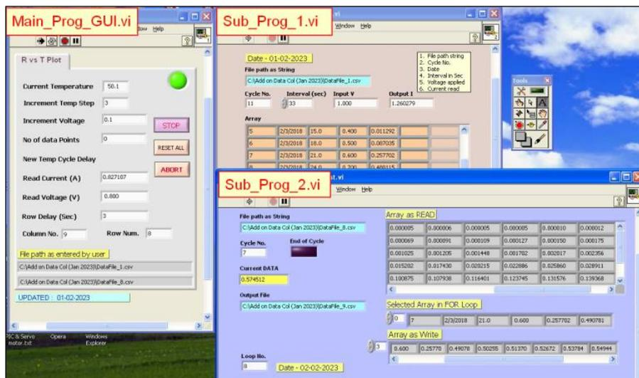
Figure 1: Screenshot of three graphical interface files among them, Main\_Prog\_GUI.vi control the parameters, and the other two display the data while acquisition is in progress.
