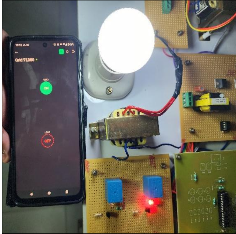
Figure 6: Proposed MCU-based EMS managed with the Blynk app. Source: Authors, (2026).
