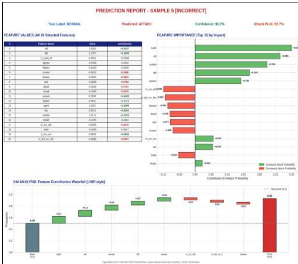
Figure 12: Demonstrates the XAI analysis for Sample-5, whereby legitimate traffic is erroneously categorized as an assault, along with feature significance and LIME-style visualizations elucidating the elements leading to the false positive prediction.
