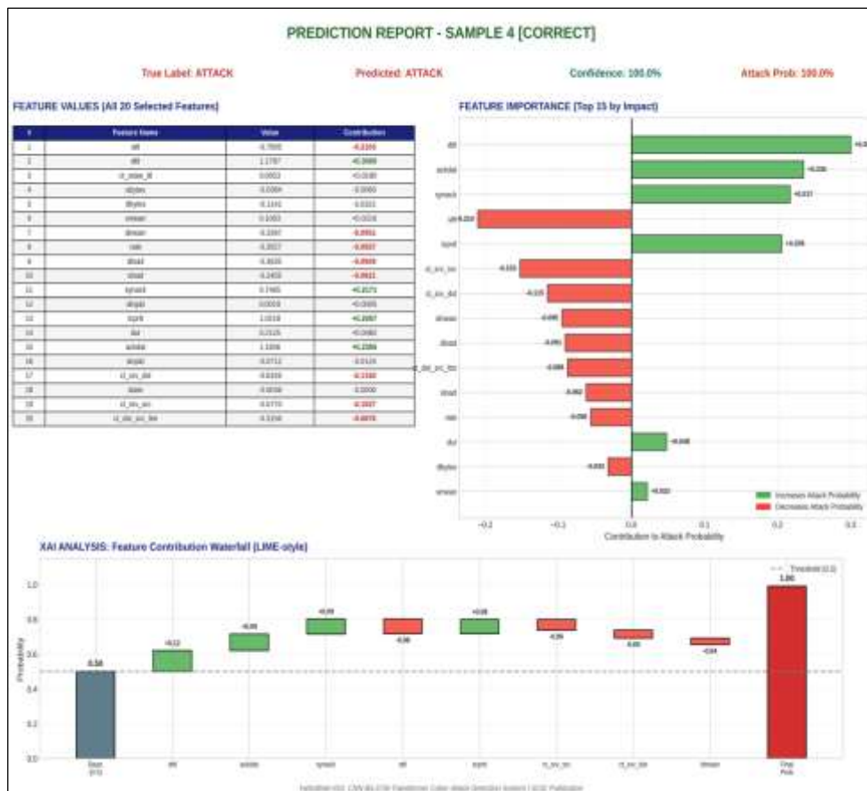
Figure 11: Provides a XAI-based analysis for Sample-4, affirming accurate attack detection with complete confidence and emphasizing the significant feature contributions that affect the final prediction.
