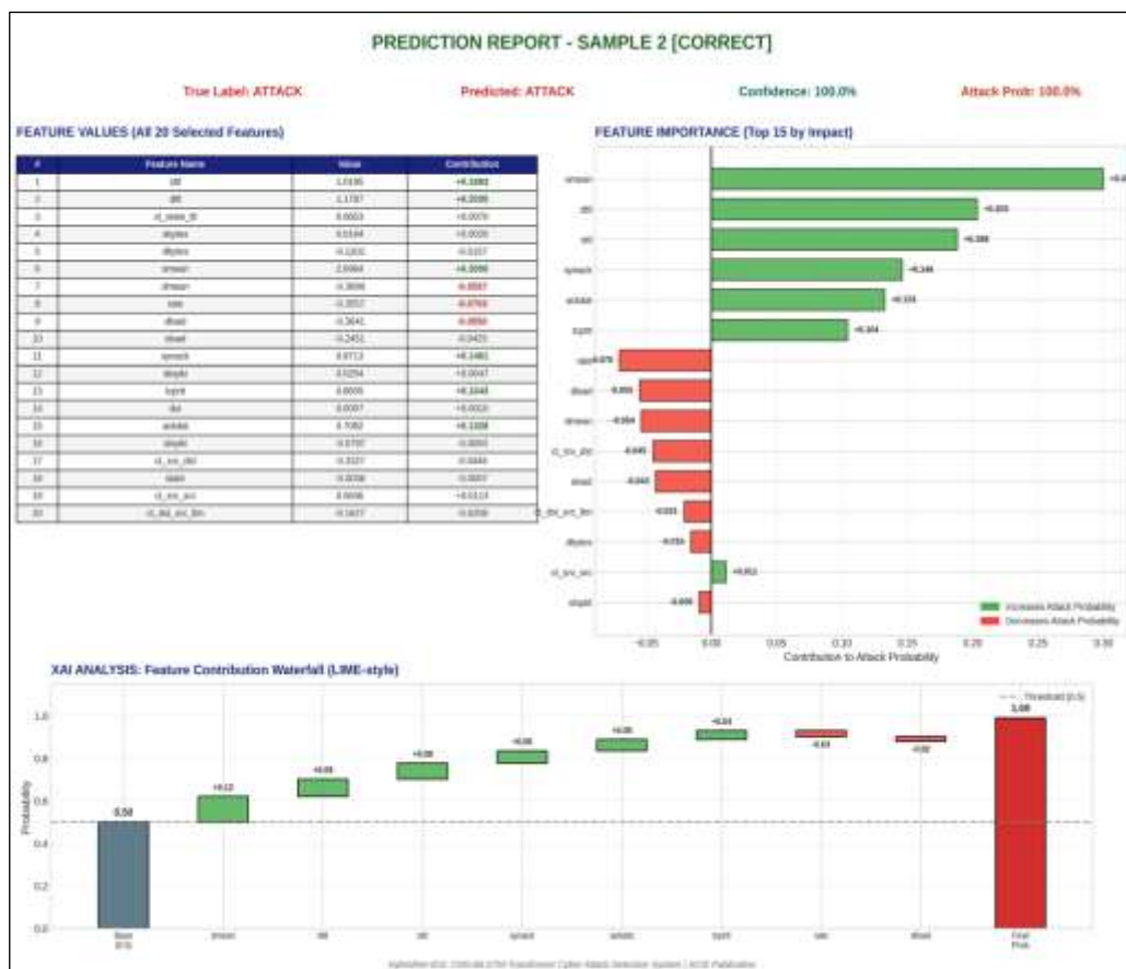
Figure 9: Displays XAI-based analysis for Sample-2, demonstrating 100% attack prediction accuracy. LIME-style waterfall graphs highlight key factors impacting the final choice. Source: Authors, (2026).
