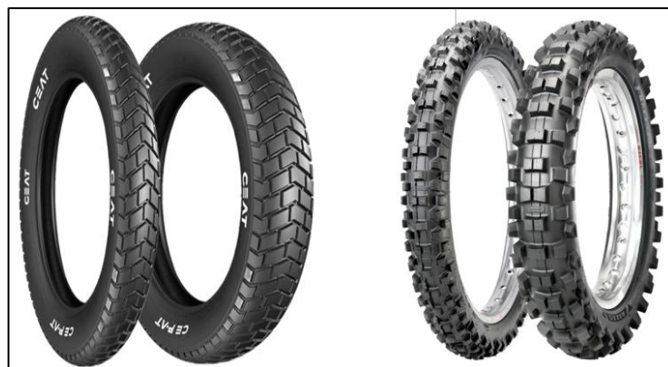
Figure 16: Tyre Shape &amp; Profile of Existing Dual Purpose &amp; Upgraded Knobby Tyres.
