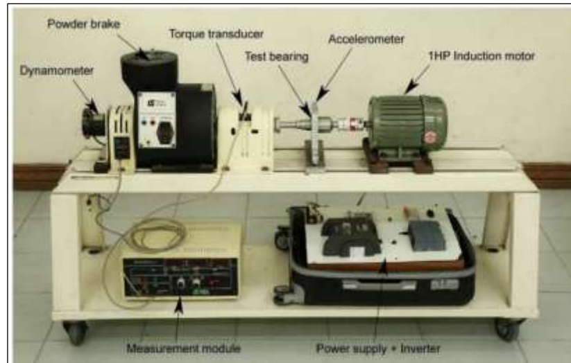
Figure 7: Practical setup for HUST bearing Test.
