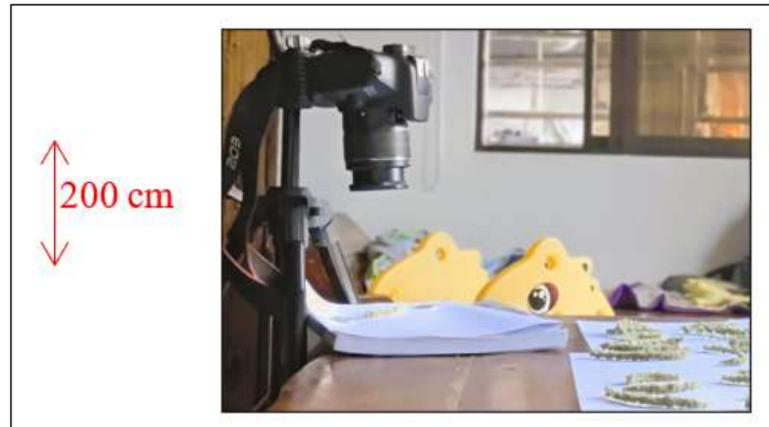
Figure 2: Camera and plant sample position for image capturing. Source: Author, (2026).
