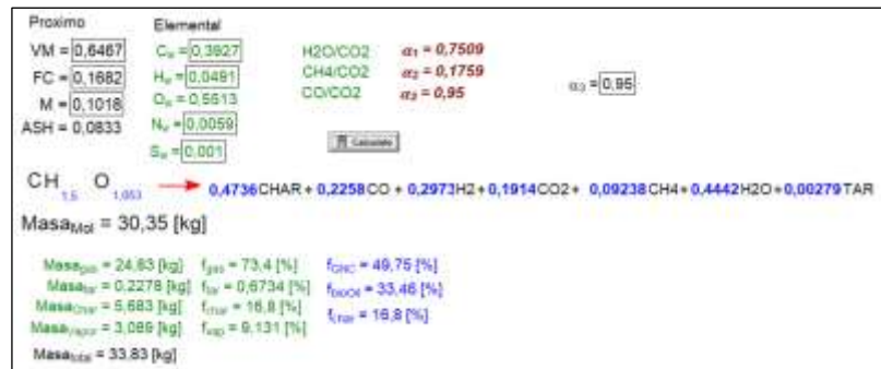
Figure 9: Pyrolysis of rice husks.
