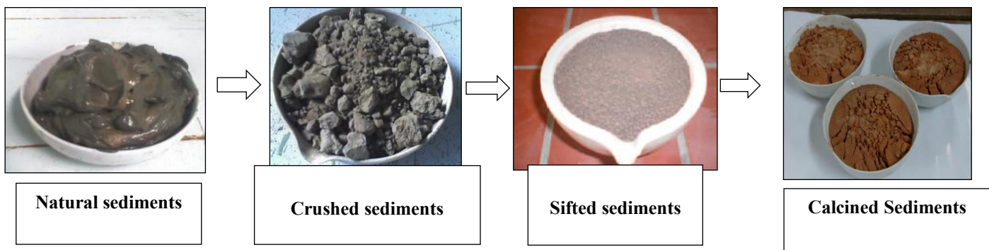
Figure 1: The calcined sediments appearance both before and after calcination.
