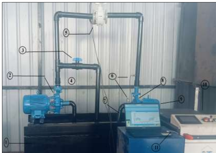
Figure 1: Experimental test setup (1) Reservoir, (2) Service pump, (3) Flow control valve, (4) Bypass line, (5) Electromagnetic flow meter, (6) Pressure transmitter, (7) Draft tube, (8) Pat, (9) DC generator, (10) Load cell, (11) DAQ.
