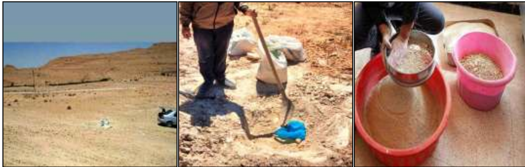
Figure 2: Process of host soil from extraction to sieving.
