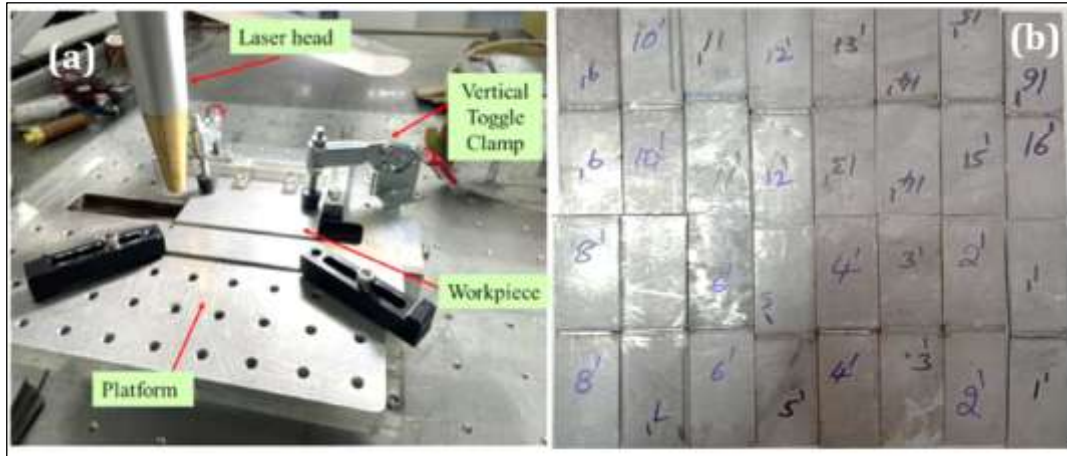
Figure 1: (a) Schematic illustration of the laser beam welding experimental setup; (b) final weldments of Ti-6Al-4V butt-joint. Source: Authors, (2026).
